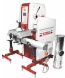
Uwira has invested in a new TEC-150-HD collar-branching machine by T-Drill, which has the ability to branch thick tubes with a wall thickness of over 10 millimeters. With this machine the amount of welded seams can be reduced. The branching
